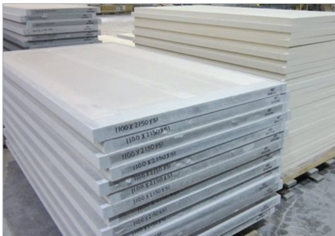
Above: Fire-rated door cores made using perlite as a lightweight functional filler.
