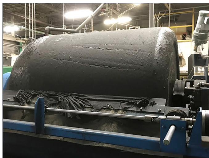
Knife removing caked solids from a drum filter septum precoat with a perlite filter aid.
